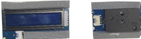
Push the feet (12) through the holes on the microcontroller board (2) stick it to the inside of the box.
